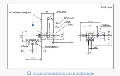
**Actuator Configuration at Front Edge**
